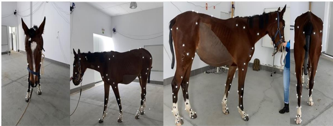
Figure 7: Representation of the set of full body markers on the horse's body. The markers selected in the highlighted markers on the left side of the horse represent the same scheme on the right side. Source: EquiPERFORM project data, January, and February 2020
